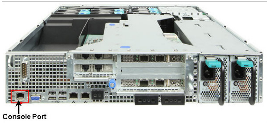
Figure 1. Location of console port
